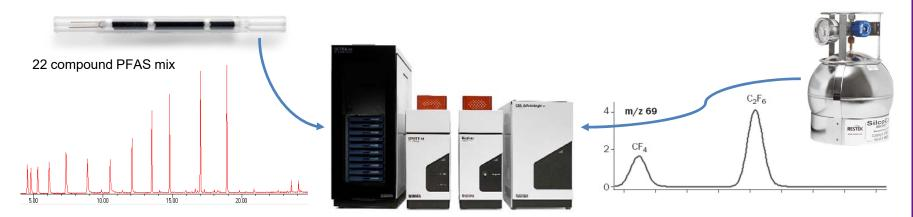
It is possible to carryout combined injection of canister and tube samples into a single injection if the samples have been co-located
